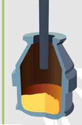
Oxygen is blown through the liquid iron and this oxidises the remaining carbon into CO and CO<sub>3</sub>. The reaction is exothermic (gives out heat) and steel scrap is added to reduce the temperature in the furnace. The molten steel is refined in a separate ladle furnace.
