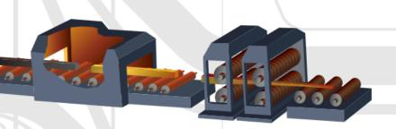
Steel is reheated and descaled before being rolled into strip/coil (from slabs), rod/bar (from billets) and sections (from blooms). The number and sequence of mill stands is matched to the thickness reduction and material properties required. Cold rolling, descaling, tempering and shearing processes can follow.
