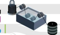
Steel is cleaned before being coated with zinc (galvanised), tin plate or a range of paints (organic coatings). This provides corrosion protection for steel outside or in demanding applications such as food cans.
