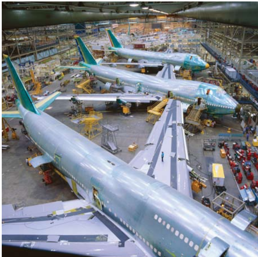
Figure 8. Boeing produces one $200 million plane per day in massive production lines that could be a model for mass production of liquid fluoride thorium reactors. Centralized mass production offers the advantages of specialization among workers, product standardization, and optimization of quality control, as inspections can be conducted by highly trained workers using installed, specialized equipment.
